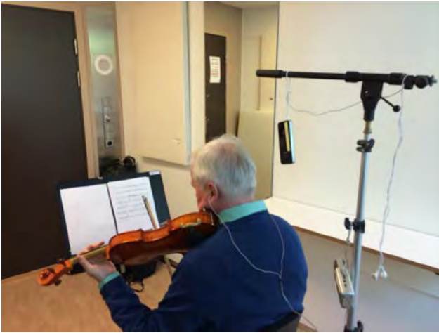
Figure 1 Individual rehearsal room, V=30\text{m}^3 ; T=0.4\text{s} ; G_{\text{rev}}(V,T)=26\text{dB}
