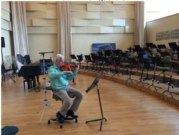
Figure 2 Big rehearsal room, intended for groups, V=1000\text{m}^3 ; T=0.8\text{s} ; G_{\text{rev}}(V,T)=14\text{dB}
